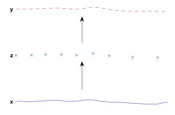
Figure 1. Example of equivalence classes of future paths for single-target sensor management. A simulated future x and a sensor scheme s to generate observations z which are input into a filter giving a track y which can be compared to x in order to evaluate s.
