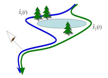
Figure 2. This figure illustrates the concept of equivalent paths. Given the sensor location shown, it is impossible to distinguish between the two paths; hence they belong to the same equivalence class.
