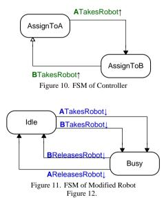
This component regulates the assignment of Robot to machines switching between them. We modify Robot to be a reactive component, which recieves ATakesRobot or BTakesRobot events from the controller, as shown in Figure 11. The PN model of the manufacturing system with added controller, obtained by BOM-to-PNML transformation, is shown in Figure 12.
