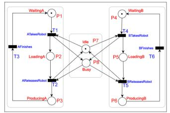
Figure 9. PN Model of the Manufacturing System
