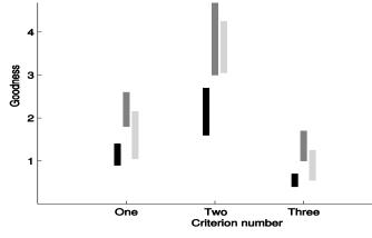
Fig. 2. A simple example with three plans (black, dark grey, light grey), and how their simulated outcomes from different seeds (giving values within a bar, indicating a *min-max* interval) fulfill three parameter criteria intervals. The two grey plans are seen to be Pareto optimal. The black plan can be filtered away after comparison with the dark grey plan.
