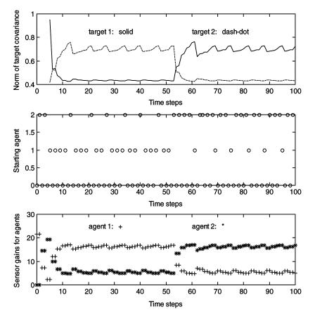
Figure 7. Covariance tuning when desired levels are not achievable simultaneously.
