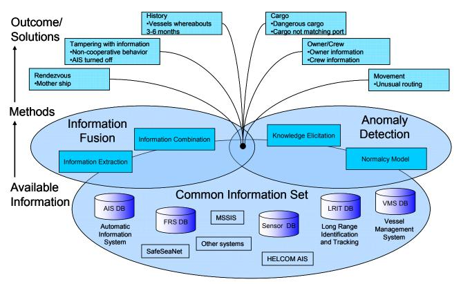
Figure 2. System architecture (Information Fusion, Anomaly Detection, and CIS)
