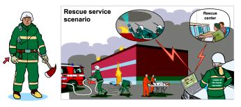
Fig. 3. In this scenario on-body sensors are primarily monitoring the vital status of fire fighters and rescue personnel in dangerous environments. Sensors can also be used to monitor the location of the individual fire fighters as well as external environment, e.g. ambient temperature, oxygen content, chemical 'sniffers' for explosive gases, etc.
