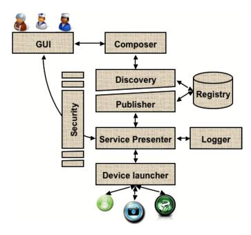
Fig. 4. Overview of the TOppS framework. Supporting C2 systems with sensor services.
