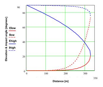
Figure 5. Elevation (solid line) and impact angle (dashed line) as function of distance. Low trajectories are red and high trajectories blue.
