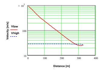
Figure 4. Velocity as a function of impact distance. The low trajectory is solid red and the high trajectory dashed blue.
