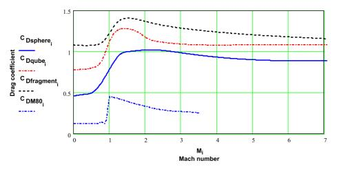
Figure 6. Aerodynamic drag coefficient for three different fragment types and M80 7.62 mm bullet.
