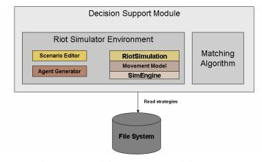
Figure 12. Decision Support Module (DSM).
