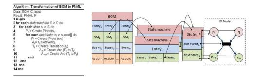
Fig. 1. a) Our Algorithm b) Transformation from BOM to PN
