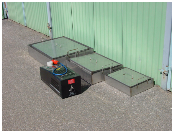
Figure 2 Smoke generator ZR-41 and fire trays A1-A3.
