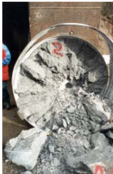
Figure D.43. Post test configuration for target 2 in test-series 1998:2. Front face.
