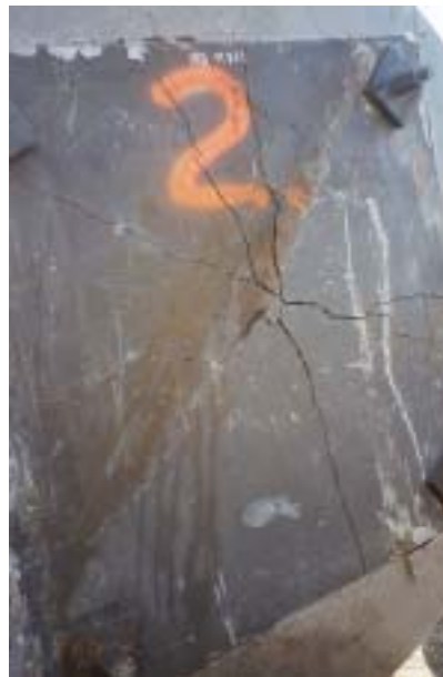
Figure D.31. Post test configuration for target 2 in test-series 1998:1. Back face.
