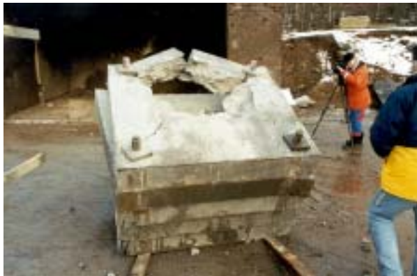
Figure D.16. Post test configuration for target 4 in test-series 1996:2. Front face. The target has been turned over by the projectile.
