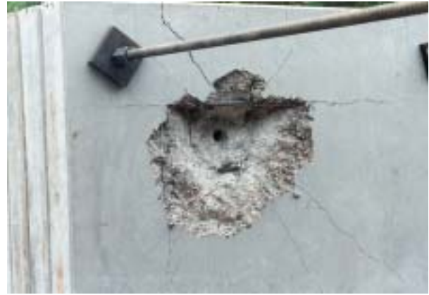
Figure D.2. Post test configuration for target 1 in test-series 1996:1. Back face.
