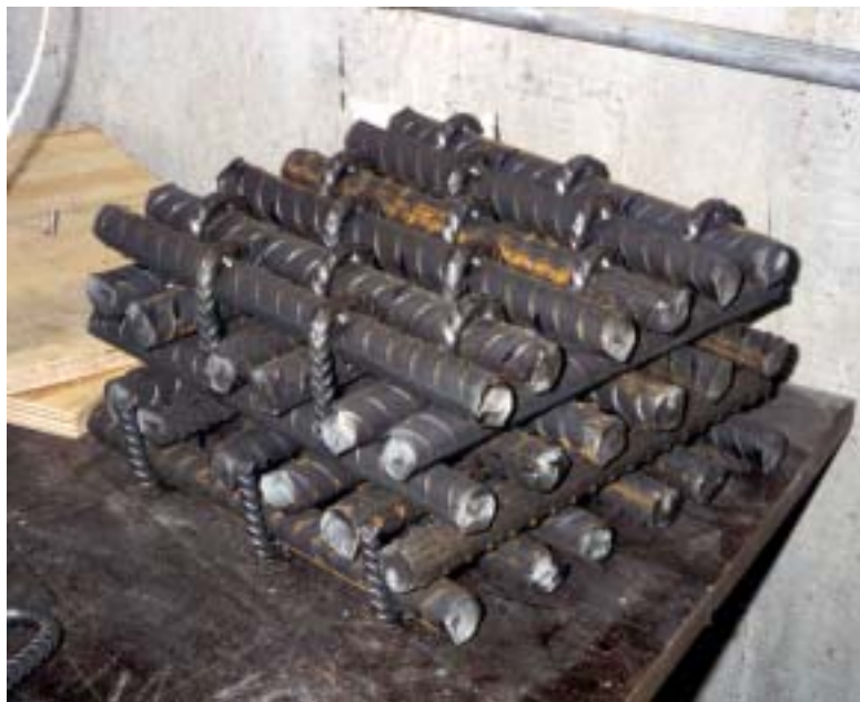
Figure 2.23 Reinforcement of CRC concrete. Volume fraction of 25 %.
