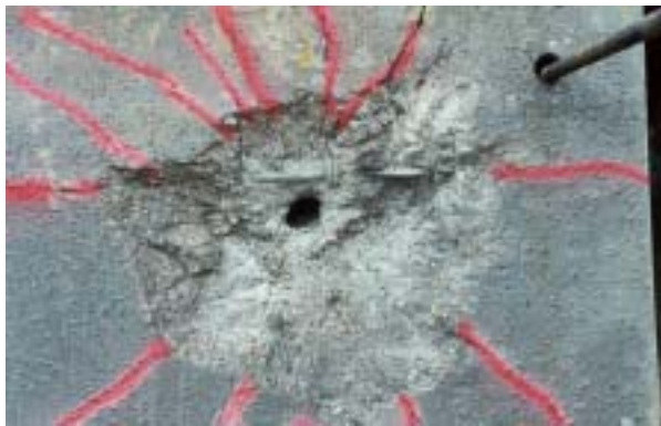
Figure D.5. Post test configuration for target 3 in test-series 1996:1. Front face shot 1.
