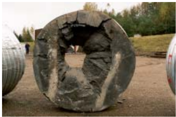
Figure D.62. Post test configuration for target 4 in test-series 1999. Back face.
