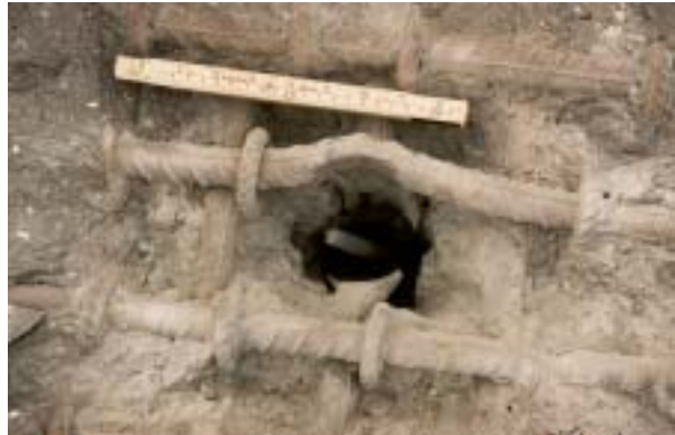
Figure D.70. Post test configuration for target 8 in test-series 1999. Front face detail.
