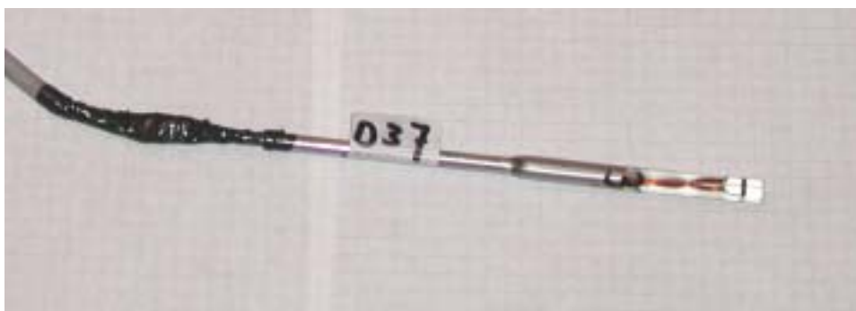
Figure 3.14 Carbon resistor pressure probe provided by TNO.
