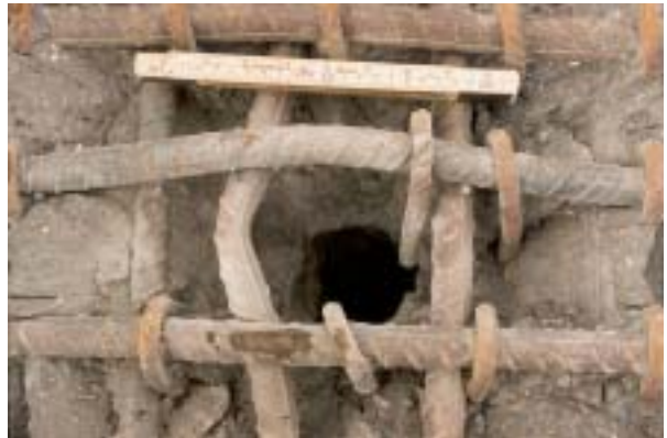
Figure D.72. Post test configuration for target 9 in test-series 1999. Front face detail.
