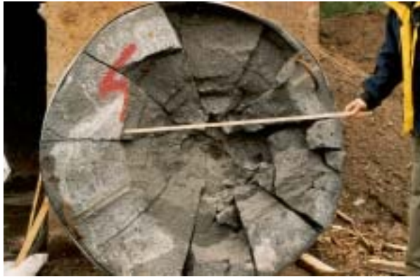
Figure D.55. Post test configuration for target 1 in test-series 1999. Front face.
