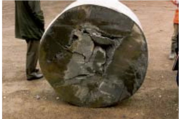
Figure D.58. Post test configuration for target 2 in test-series 1999. Back face.
