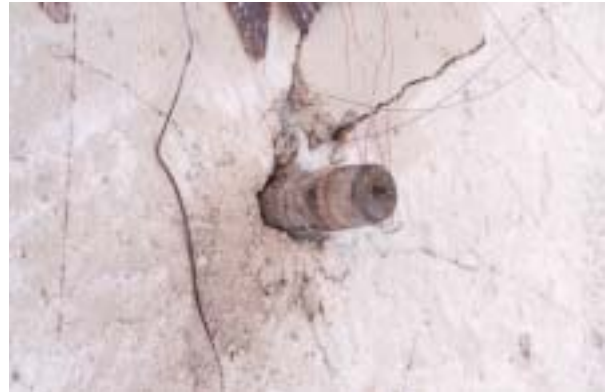
Figure D.20. Post test configuration for target 1 in test-series 1997. Projectile stuck in target plate 4.
