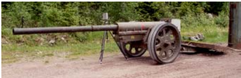
Figure 3.2 The 105-mm calibre gun and Doppler radar used for test series 1996:1.
