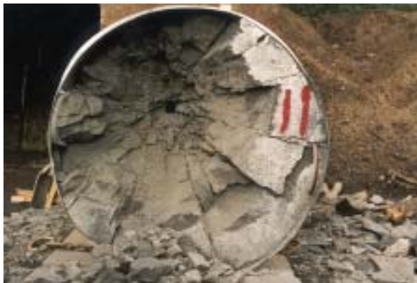
Figure D.75. Post test configuration for target 11 in test-series 1999. Front face.
