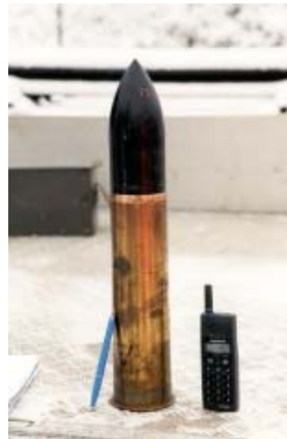
Figure 3.8 The 75-mm-calibre gun and the 75-mm-calibre armour-piercing projectile and case used in test series 1997.
