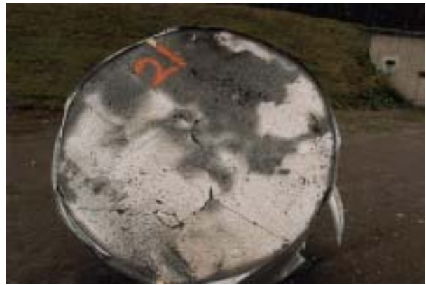
Figure D.92. Post test configuration for target 19 in test-series 1999. Back face.
