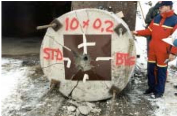
Figure D.19. Post test configuration for target 1 in test-series 1997. Front face.
