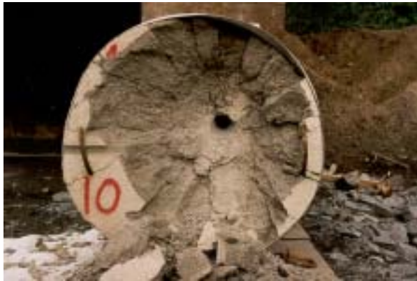
Figure D.73. Post test configuration for target 10 in test-series 1999. Front face.
