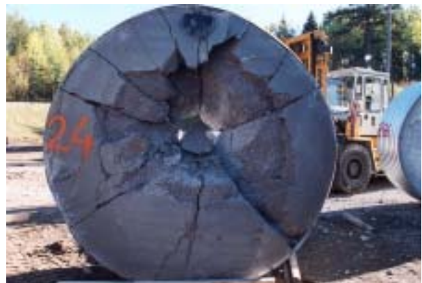
Figure D.104. Post test configuration for target 24 in test-series 1999. Back face.
