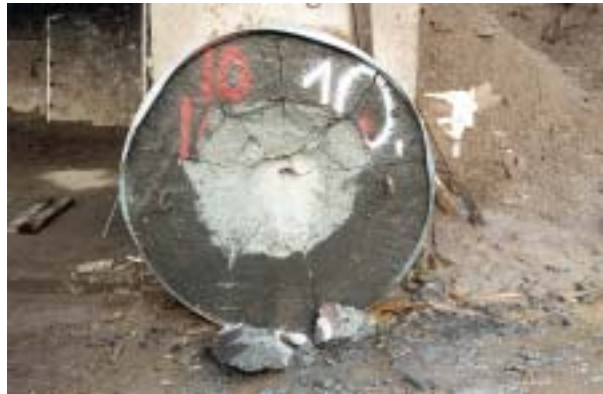
Figure D.51. Post test configuration for target 10 in test-series 1998:2. Front face.
