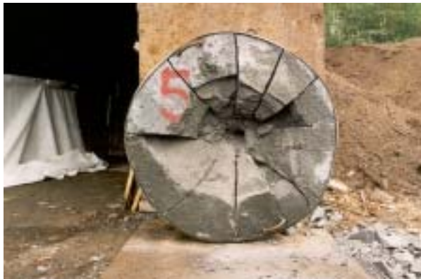
Figure D.57. Post test configuration for target 2 in test-series 1999. Front face.
