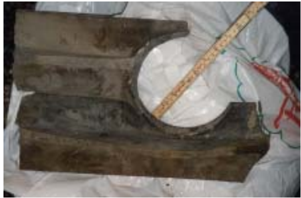
Figure D.95. Post test configuration for target 10 in test-series 1999. Hole in the steel rail reinforcement made by the projectile .
