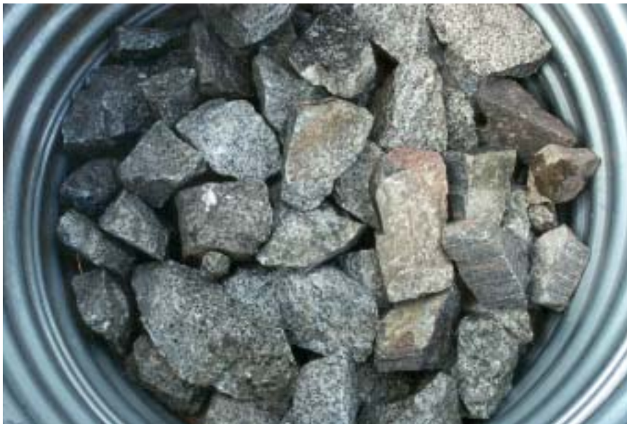
Figure 2.25 Target 19 of test series 1999. Rock boulders measuring 200 – 400 mm across.
