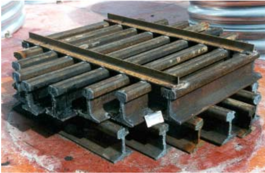
Figure 2.24 Target 20 in test series 1999. The rails are welded together.
