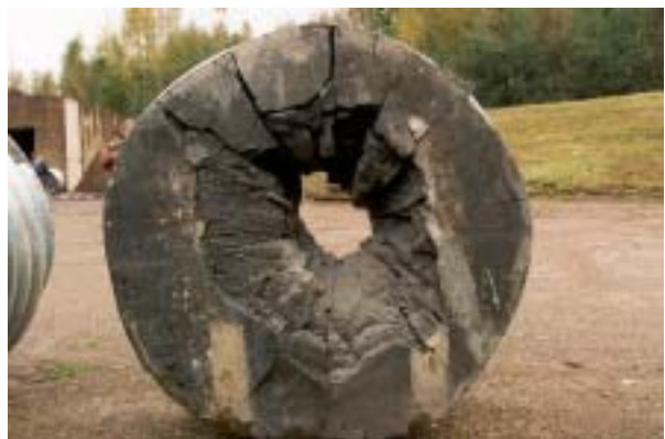
Figure D.66. Post test configuration for target 6 in test-series 1999. Back face.
