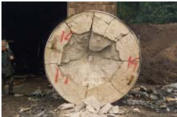
Figure D.81. Post test configuration for target 14 in test-series 1999. Front face.
