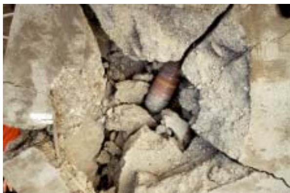
Figure D.18. Post test configuration for target 4 in test-series 1996:2. Front view of projectile inside target.
