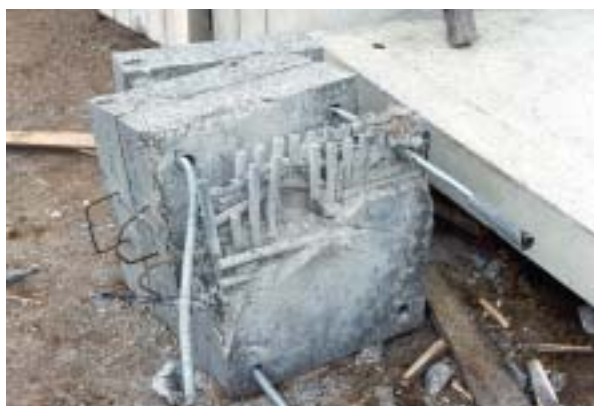
Figure D.9. Post test configuration for target 4 in test-series 1996:1. Top front face.
