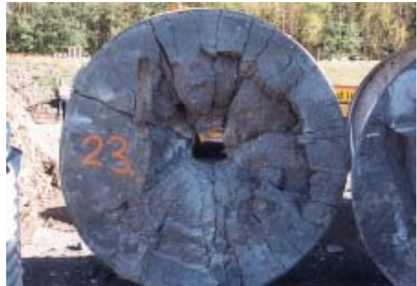
Figure D.101. Post test configuration for target 23 in test-series 1999. Back face.
