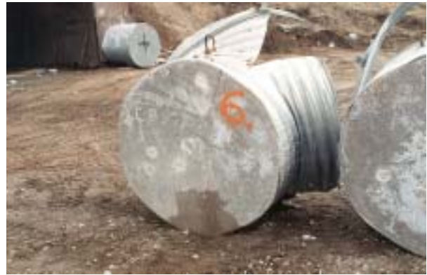
Figure D.36. Post test configuration for target 6 in test-series 1998:1. Front face. Figure D.37. Post test configuration for target 6 in test-series 1998:1. Back face.
