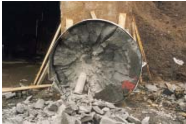
Figure D.85. Post test configuration for target 16 in test-series 1999. Front face.
