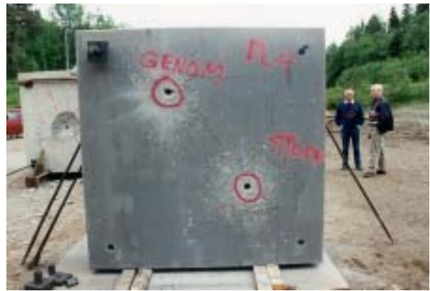
Figure D.6. Post test configuration for target 3 in test-series 1996:1. Back face of target plate 4.
