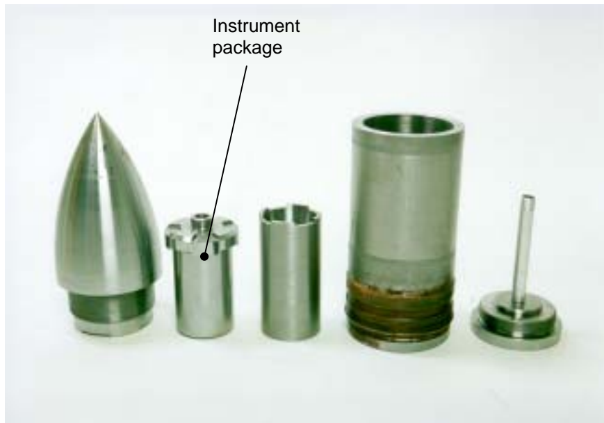
Figure 3.13 Disassembled modified 152 mm-calibre projectile used in test-series 1999.
