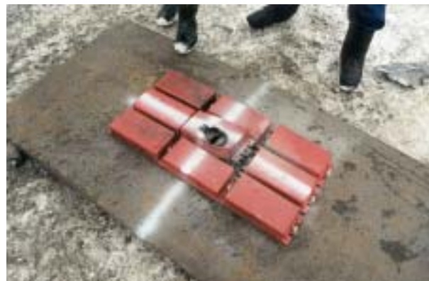
Figure D.22. Post test configuration for target 2 in test-series 1997. Front face of ERA-panel.
