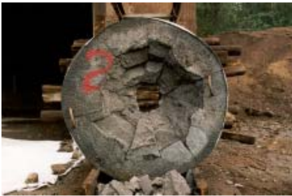
Figure D.63. Post test configuration for target 5 in test-series 1999. Front face.
