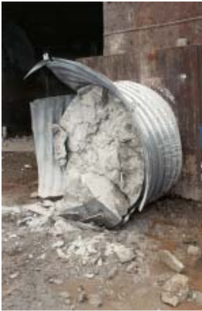
Figure D.36. Post test configuration for target 6 in test-series 1998:1. Front face. Figure D.37. Post test configuration for target 6 in test-series 1998:1. Back face.
