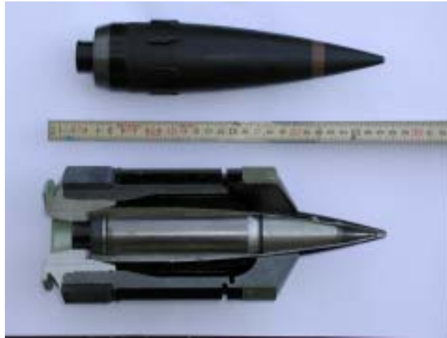
Figure 3.3 The 57-mm-calibre armour-piercing sabot discarding projectile with a 43 mm-calibre penetrator used in test series 1996:1.
