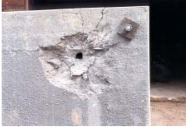
Figure D.1. Post test configuration for target 1 in test-series 1996:1. Front face.
