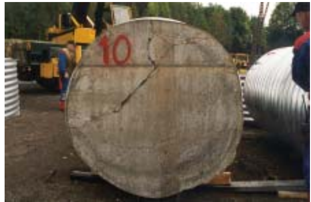
Figure D.74. Post test configuration for target 10 in test-series 1999. Back face.
