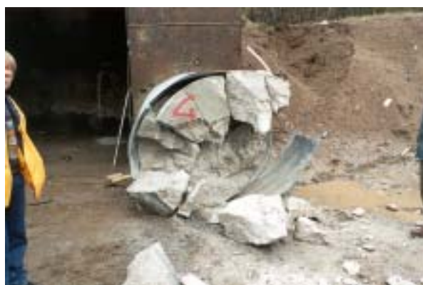
Figure D.45. Post test configuration for target 4 in test-series 1998:2. Front face.
