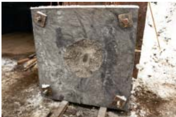
Figure D.21. Post test configuration for target 2 in test-series 1997. Front face.
