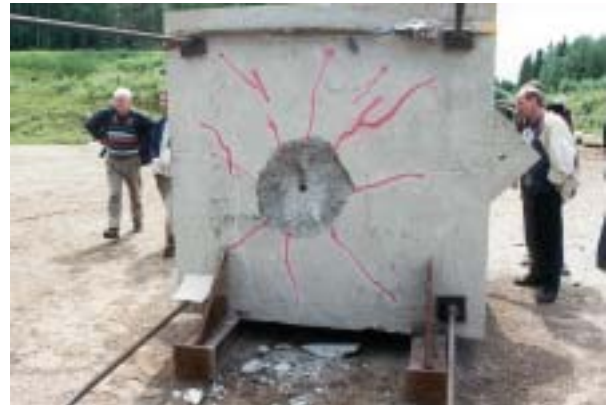
Figure D.4. Post test configuration for target 2 in test-series 1996:1. Back face.
