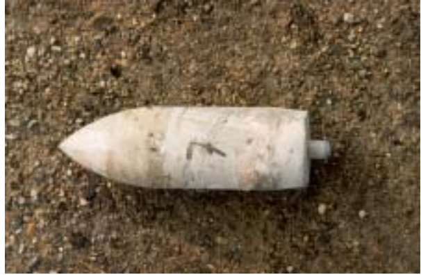
Figure D.68. Post test configuration for target 7 in test-series 1999. Projectile.
