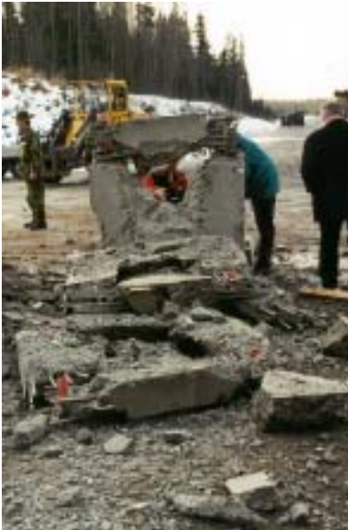
Figure D.12. Post test configuration for target 2 in test-series 1996:2. Back face.
