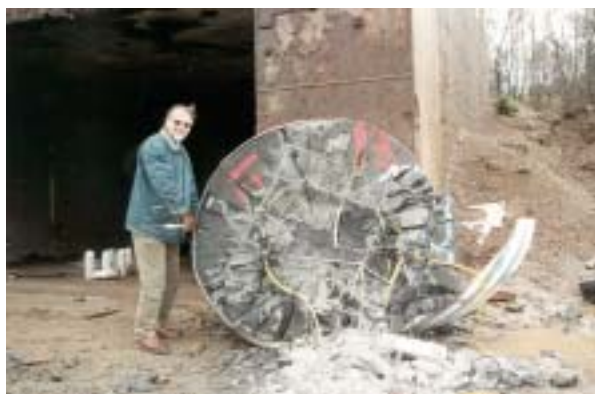
Figure D.54. Post test configuration for target 13 in test-series 1998:2. Front face.
