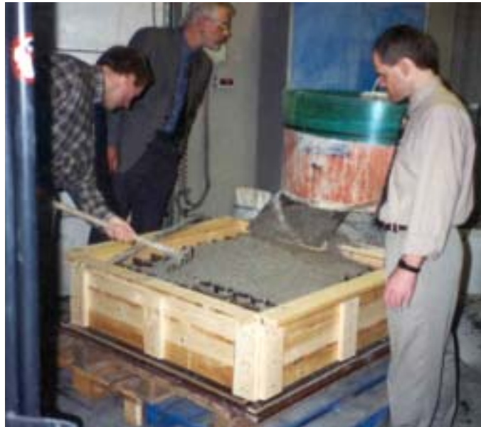
Figure 2.6 Casting of CRC concrete at Densit A/S in February 1997.
