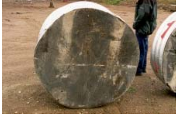
Figure D.56. Post test configuration for target 1 in test-series 1999. Back face.
