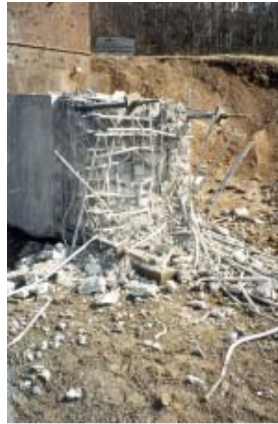
Figure D.33. Post test configuration for target 4 in test-series 1998:1. Front face.
