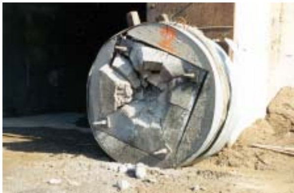
Figure D.30. Post test configuration for target 2 in test-series 1998:1. Front face.
