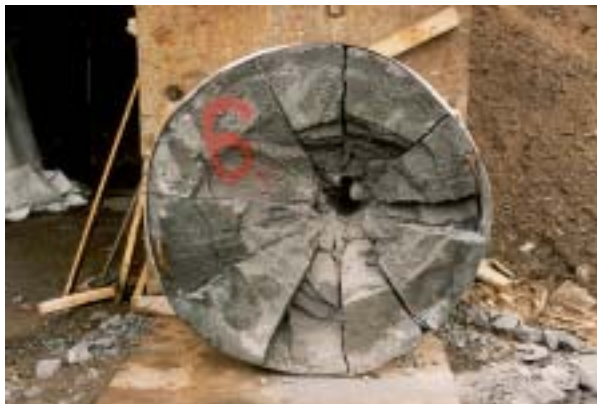
Figure D.59. Post test configuration for target 3 in test-series 1999. Front face.
