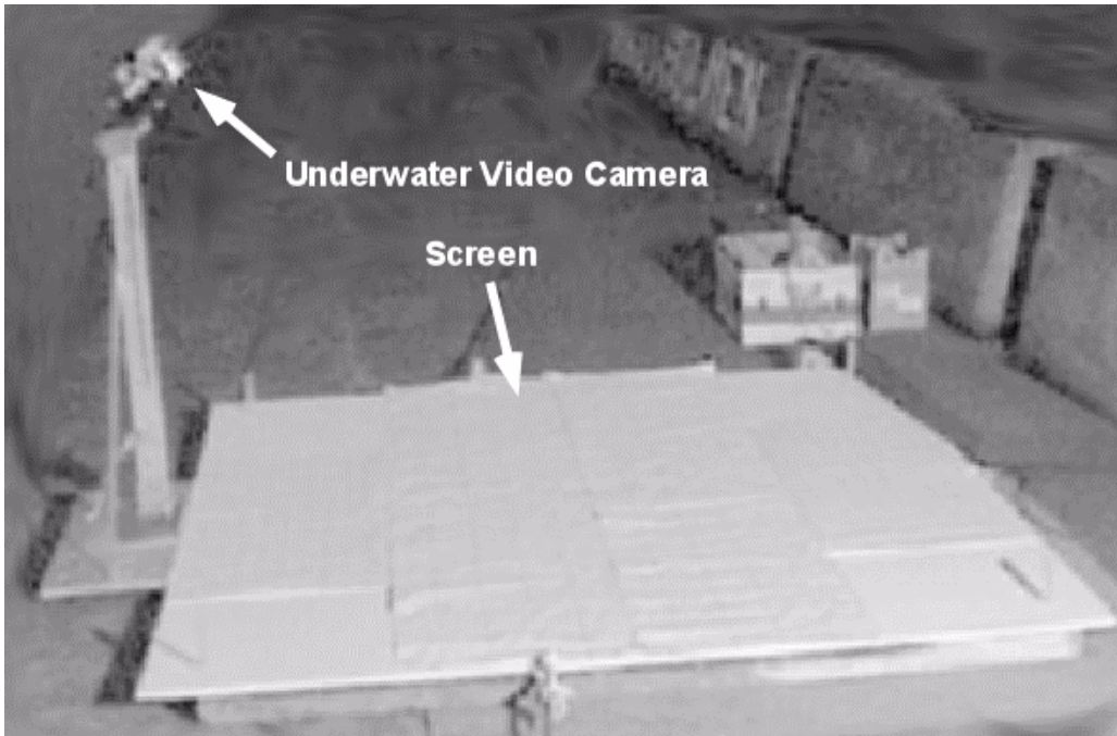
Figure 1. The beam profile screen with attached underwater video camera.
