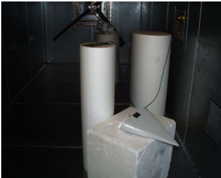
Fig. 1. Measurement of microwave coupling to a PCB in the reverberation chamber at FOI. The dimensions of the RC is 5.10 m * 2.46 m * 3.00 m. In the foreground the transmitting antenna is seen. The PCB is on top of the left styrofoam cylinder.
