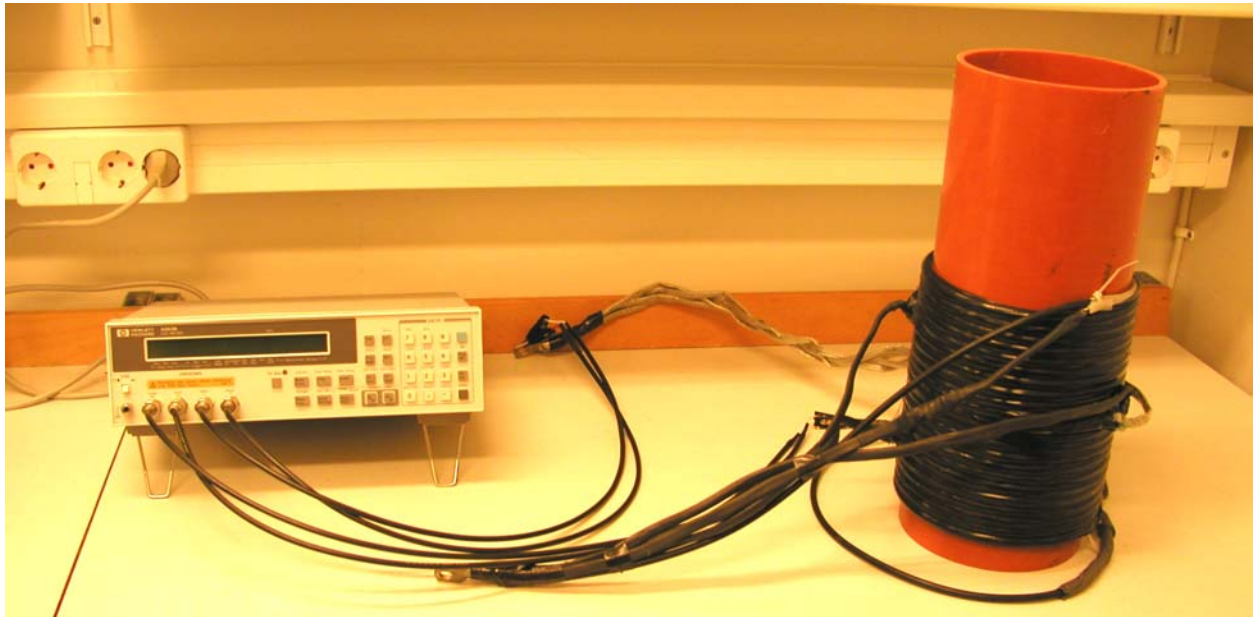
Figure 24. Inductance measurement of semicon transformer.
