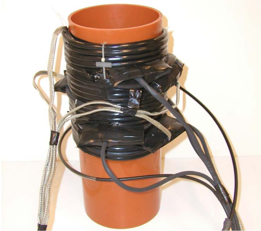
Figure 48. Modified transformer with rubber insulated terminals.
