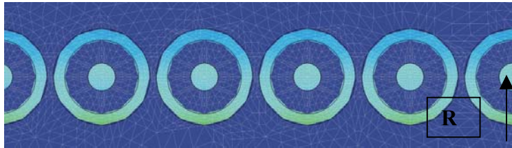
Figure 36. Simulation of current density in solenoidal cross section at 1 kHz.
