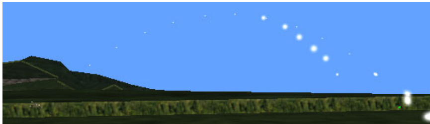
Figure 9 V_{exp}[0-1.0] set to 1.0 means that the flares gets the expendables initial speed when released. Small dots show the trajectory of the expendable and larger dots show the trajectory of the flare.
