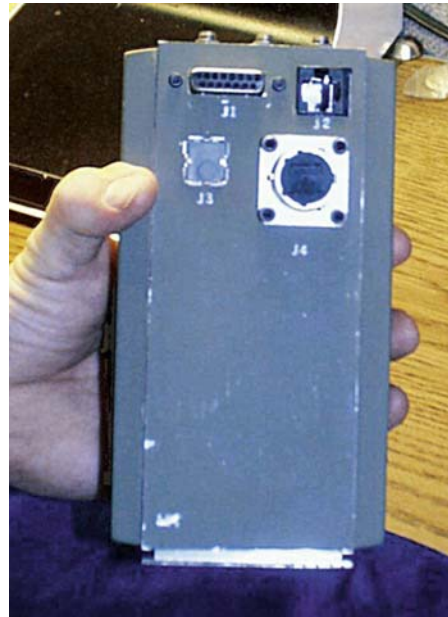
Figure 2.6: Early ITT design goal for the SUO – SAS system. All the components in a 1.5 kg box, including battery, but its realization falls outside DARPA's project. Source: [13].
