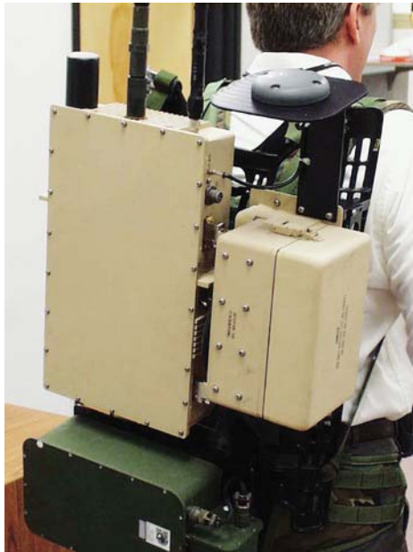
Figure 2.5: ITT SUO - SAS prototype. The flat box on the left is the radio and computer with three antennas on top. The bulky box on the right is the battery box and the box below is the geo-location system with its flat circular antenna above the battery box. Source: [13].
