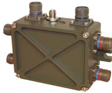
Figure 2.3: SAAB SRR360 access point transceiver. Source: [6].
