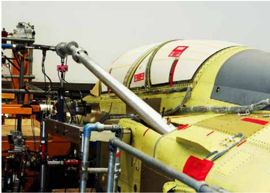
Figure 7. Photograph of the forward fuselage, D version, with the air-to-air refuelling probe dummy.
