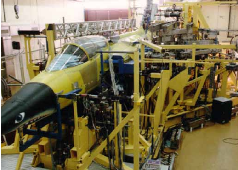
Figure 5. Photograph of the full scale fatigue test of the Gripen single seater, 39A.
