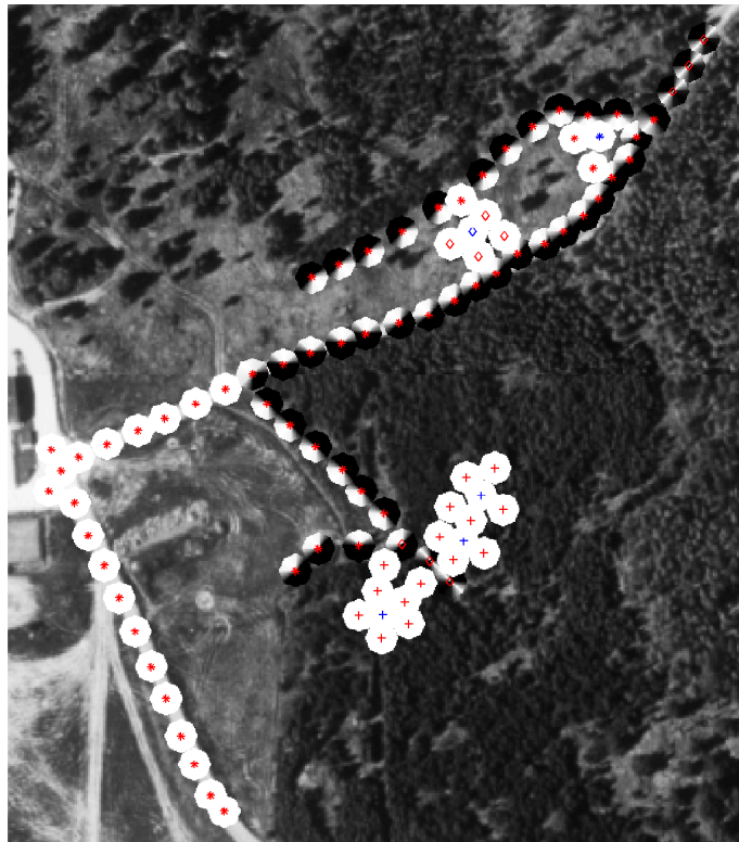
Figure 10.7: Road and objects surveillance scenario. Feature positions and their occlusion symbols. Plus, diamond and star signs represent short, medium, long maximum range, respectively.
