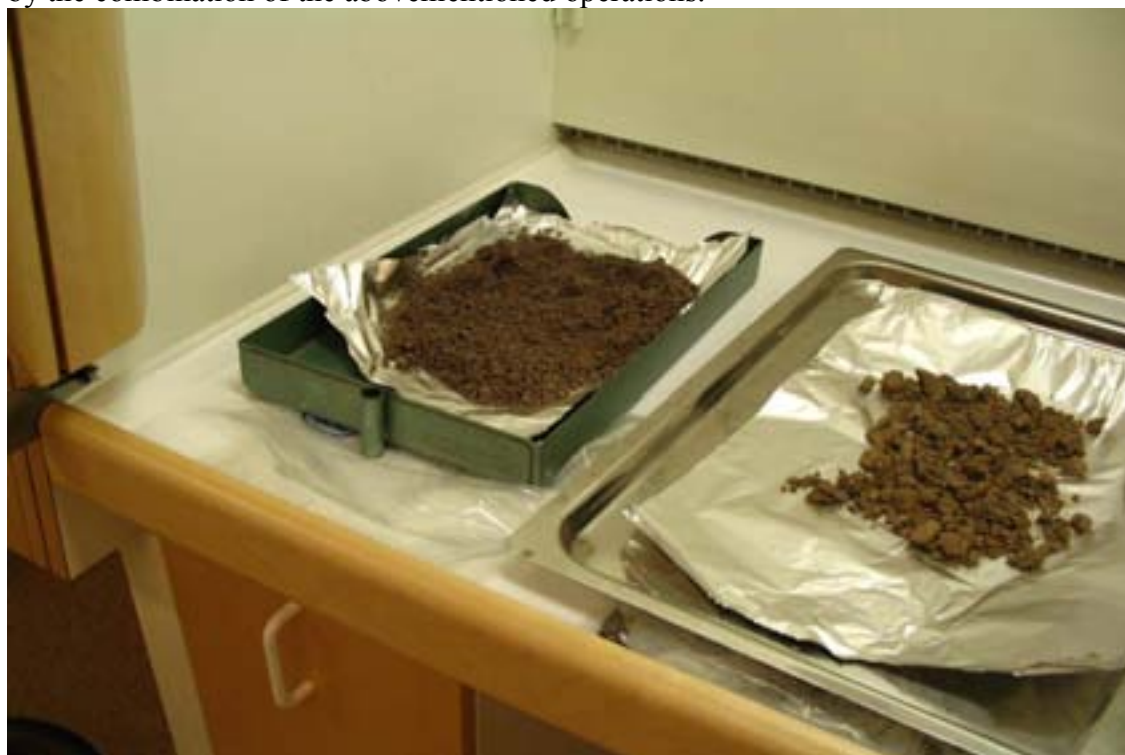
Figure 1. Samples were dried and larger crystalline objects were removed before sieving and milling.
