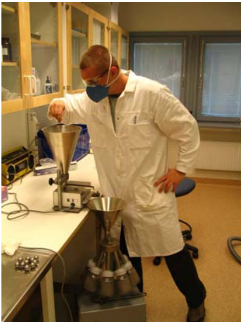
Figure 3. The samples were loaded into a stationary feeder with a vibrating conveyer connected to a sectorial splitter.
