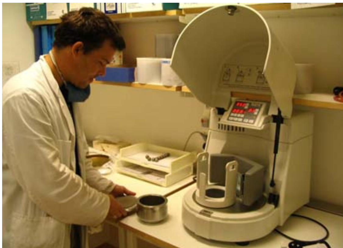
Figure 2. A ball mill (Planetary Mono Mill) equipped with a stainless steel bowl in which sample and grinding balls were put.
