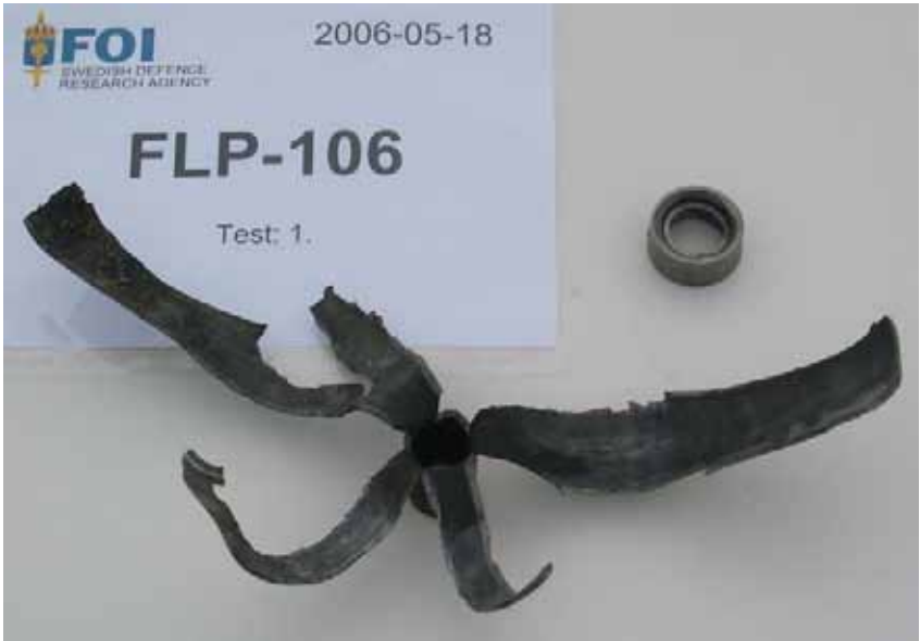
Figure 3. Results from the 25 mm detonation test, DN 25 [20].
