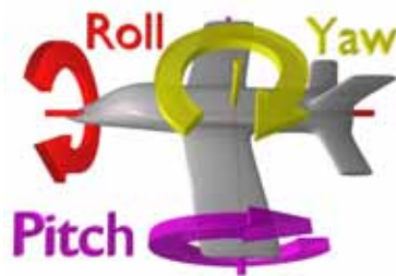
Figure 3.3: The three rotational degrees of freedom in an aircraft. This image is licensed under the GNU Free Documentation License, http://en.wikipedia.org/wiki/Image:Flight_dynamics.jpg
