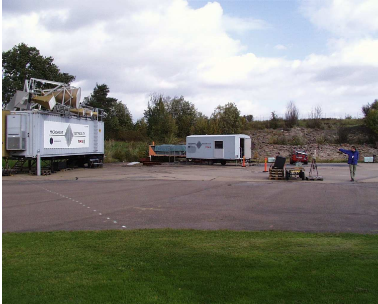
Figure 1.1: A typical radiated susceptibility test (RST) at an open area test site (OATS). The Swedish microwave test facility (MTF), on the left side of the picture, generates a strong electromagnetic plane wave which hit the equipment under test (EUT), on the right side of the picture. It is concluded whether the EUT can withstand a certain test level or not.
