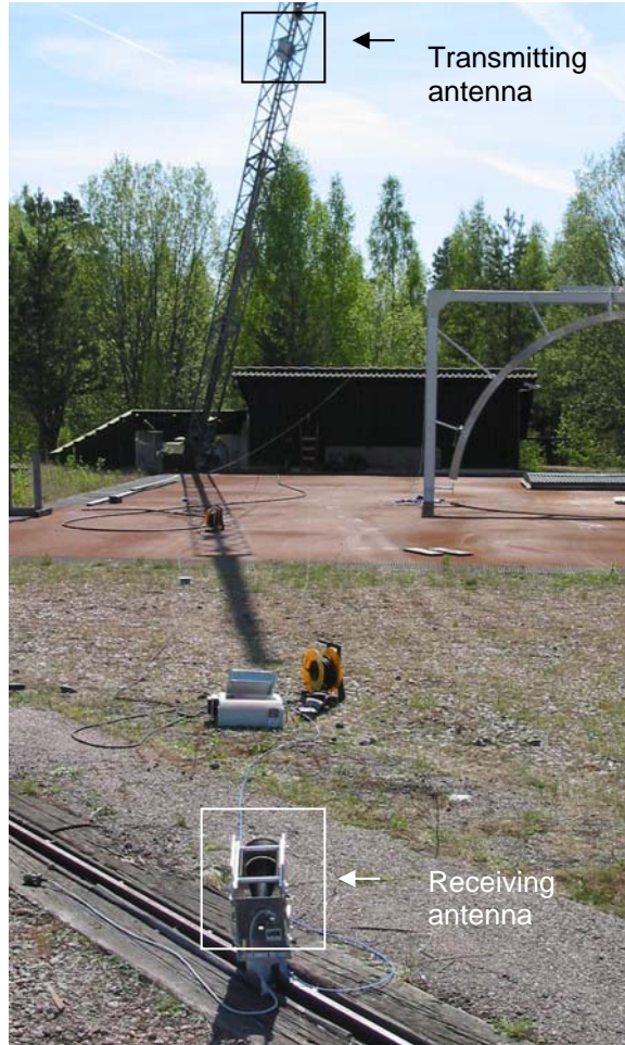
Figure 10. The receiving antenna is mounted on ground and directed to the transmitting antenna on the tilted tower.
