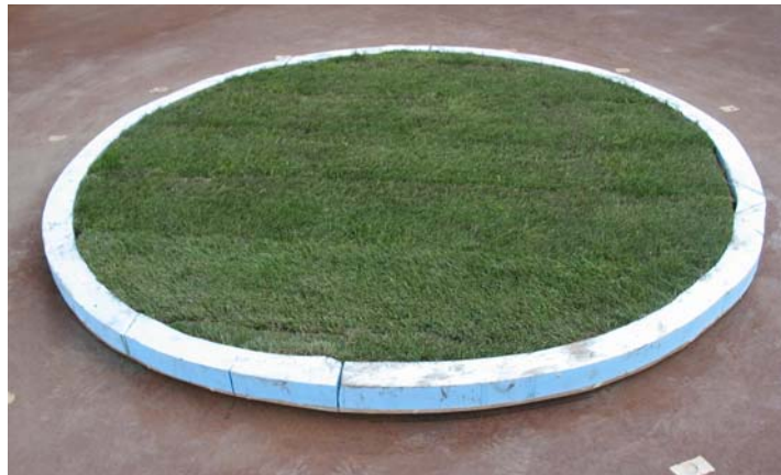
Figure 7. The circular wooden disc with polystyrene border placed on the turntable. The disc diameter is 2.45 meters. The grass is placed in two layers on the disc.
