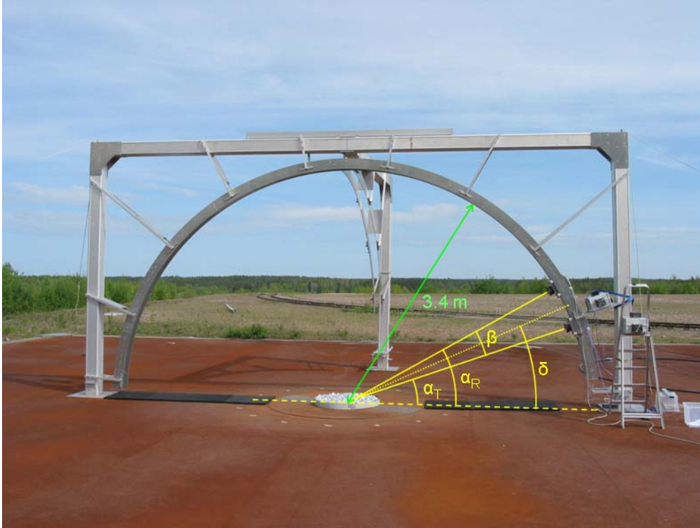
Figure 3. The bistatic arc has an inner radius of 3.4 m and can carry antenna wagons that can be moved independent of each other. Also marked are nominal angles in the plane of incidence, the transmitter and receiver depression angles, \alpha_T and \alpha_R , the bistatic angle, \beta , and the bisector depression angle \delta . Quantities used to describe local scattering geometries are defined mathematically in appendix C.
