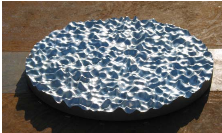
Figure 6. The rough PEC surface. The diameter is 0.9 meter.
