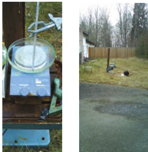
Figure 9: To the left; Resonance Raman signal from outdoor measurement on nitromethane in vapor phase at an irradiation wavelength of 220 nm. The nitromethane temperature was approximately 328 K (55°C) and the outdoor temperature was 274 K. The spectrum is accumulated from 1000 laser pulses, i.e. in 100 seconds. The two images to the right; a close up of the open NM container, and the container as seen from the lab.
