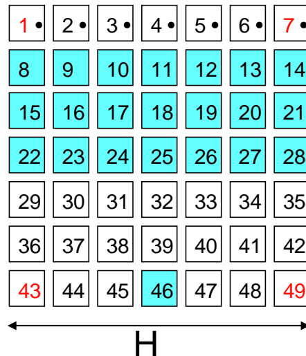
Figure 18 Array position 5. H-polarized elements, probe to the right. Subarray seen from outside. Measured elements blue.
