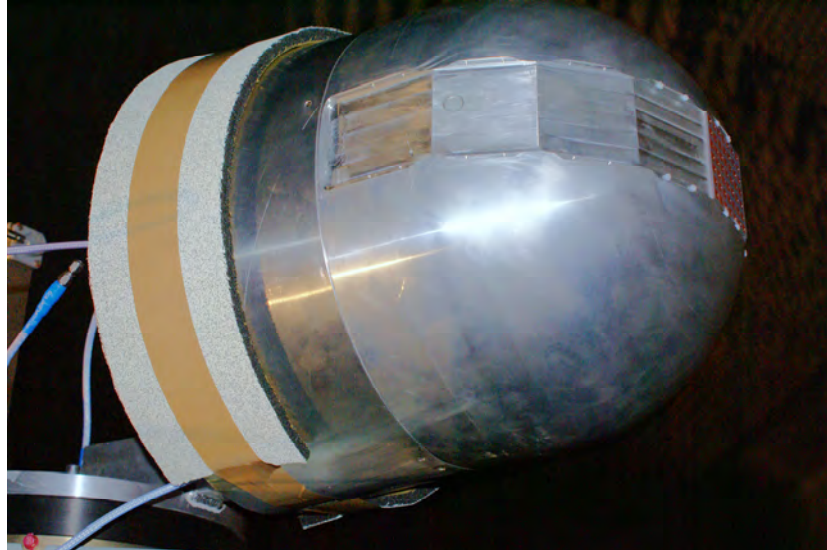
Figure 3 The right hand side, without antenna elements, with absorber shown.
