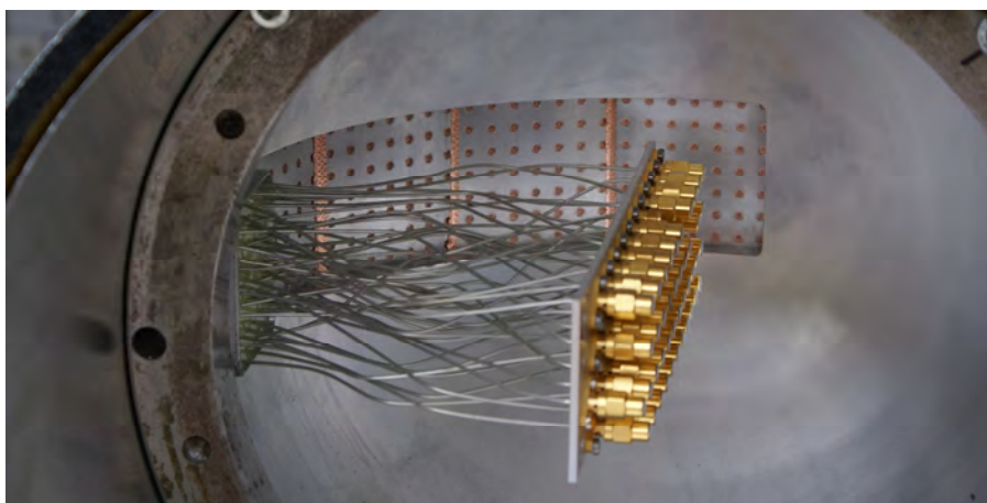
Figure 12 One active and four passive subarrays seen from the back side when measuring subarray position 5. Two elements measured and 43 terminated by coaxial load and 200 by 50 \Omega chip resistors.
