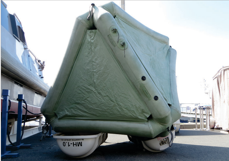
Figure 28: The Ugolok radar decoy. Source: The Swedish Defence Research Agency.
