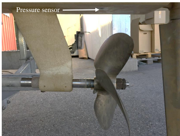
Figure 4. Pressure sensor in the hull of Eelex 8000 above the propeller, see white arrow. Photo © Kongsberg.
