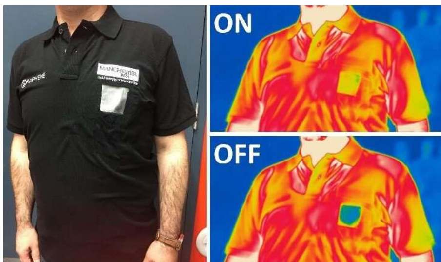
Figur 4. Textil med anpassningsbara termiska egenskaper baserat på grafen. Reprinted with permission from S. M. Ergoktas et al. , Graphene-Enabled Adaptive Infrared Textiles , Nano Letters 20(7), pp.5346-5352 (2020). Copyright 2021 American Chemical Society.
