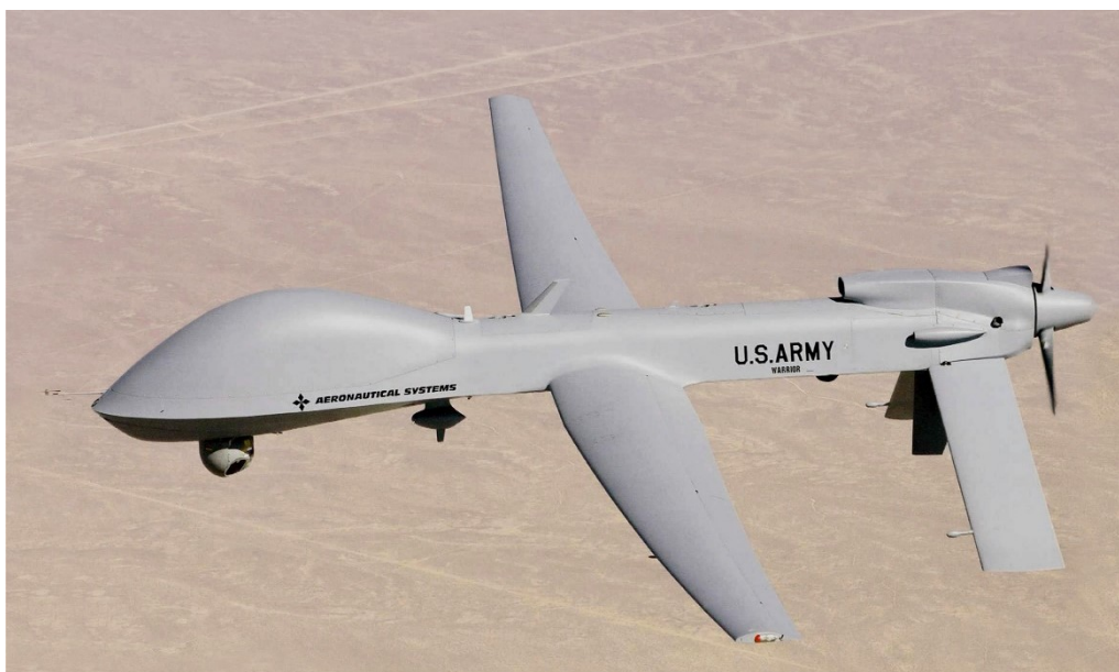
Figure 7 MQ-1C Gray Eagle. General Atomics, USA. (Photo Courtesy of U.S. Army; public domain)
